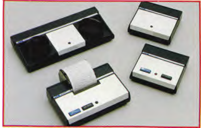
Photo 4: Four peripherals for the Telecomputer (clockwise from upper left): an acoustic interface (not the same as an acoustic coupler because the modem circuitry is already contained inside the terminal); the RS-232C interface, a video interface; and a 20-column printer.
