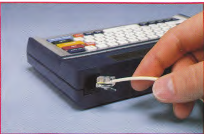
Photo 3: The FCC-registered Telecomputer is designed to attach directly to a phone using a standard modular jack. When in use, the terminal draws all of its power from the phone line.
