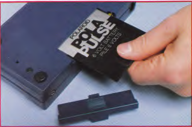
Photo 2: The Telecomputer is powered by a built-in Polaroid Polapulse flat battery.
